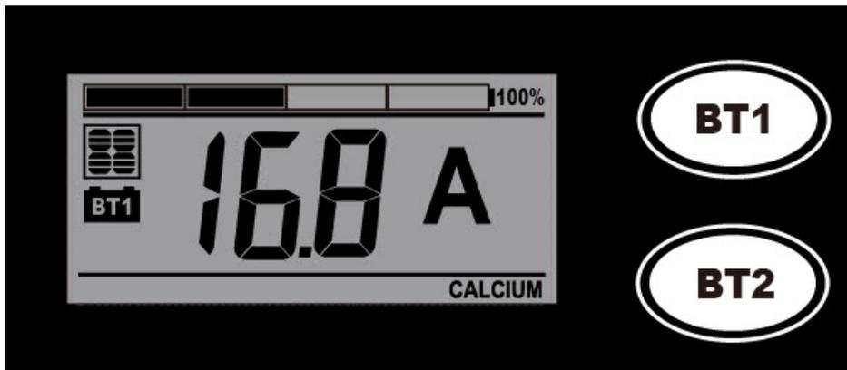
**Charging priority setting:** The dual battery controller provides the priority charging setting for Battery 1# and Battery 2#; the user can select the percentage of available charge current to each battery.
